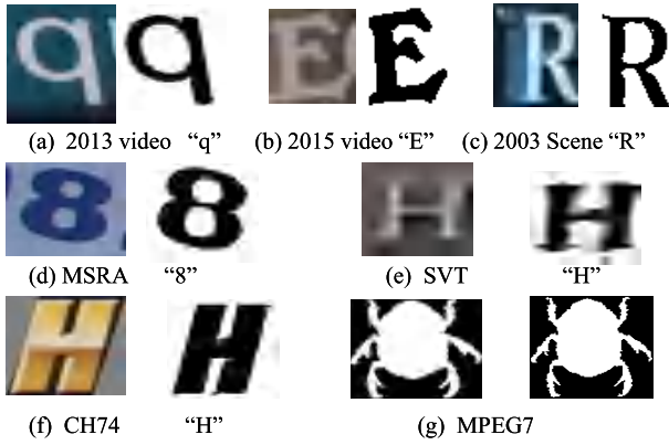
Fig. 11. Sample contour-restored results of the proposed method and respective recognition results for the different datasets. Note: Since there is no OCR available for MPEG data, recognition results are not provided. (a) 2013 video “q”. (b) 2015 video “E”. (c) 2003 Scene “R”. (d) MSRA “8”. (e) SVT “H”. (f) CH74 “H”. (g) MPEG7.
